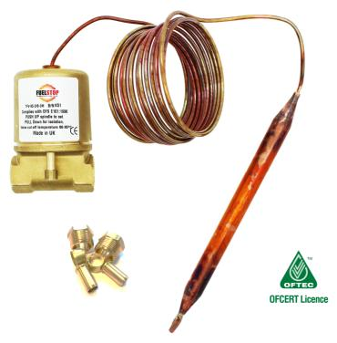
The reset button can be used as an isolation valve when the burner is being serviced by pulling the button down but must be pressed up to activate the valve into the open position before the burner is fired up.
