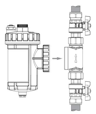
Present the filter to the connector block ensuring the air bleed is at the top and the drain plug is at the bottom. Gently push the filter into the connector block and when you are satisfied with the position of the filter, hand tighten the filter pot connecting nut. If further tightening is required, gentle pressure can be applied with a suitably sized set of pump pliers.
