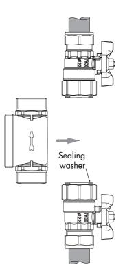
Slip the connector block between the isolation valves, taking particular care to ensure that the directional arrow on the connector block is pointing in the direction of the flow of water. Failure to do so will result in reduced flow and inhibited filter performance.
