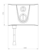
Outer Casing Easy clean, high impact polycarbonate/ ABS
