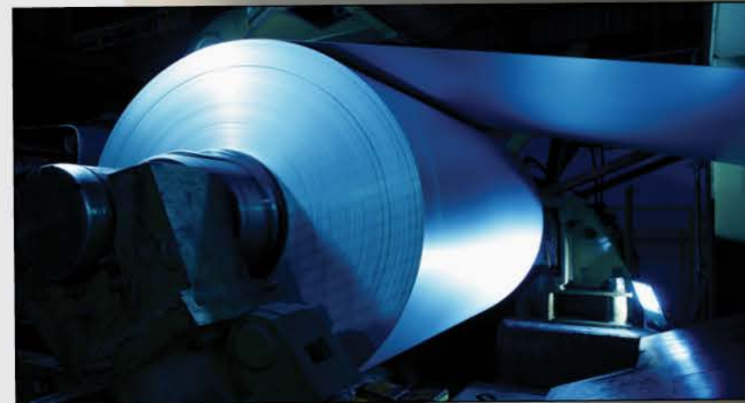
Stainless steel roll feeding spiral weld
