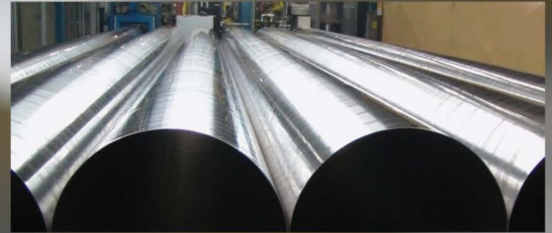
Stainless steel spiral welded tubes waiting to be laser cut into different sized cylinders
