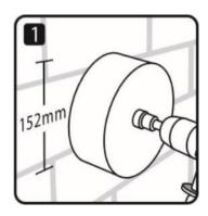
Core drill hole using standard 152mm core
