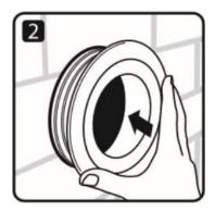
Insert PipeSnug into core-drilled hole
