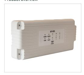
The KF-510 is a well sized robust design, with 6 zones as standard, a volt free boiler interlock and an adjustable pump delay, this product adds better performance capability to your underfloor heating system. Integrated connections for two independent valves, typically hot water cylinder and 1st floor radiator circuits, making heating controls installation easier and faster. Typically these can be two or three port zone valves
