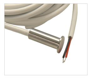
BP-260 is a multi use temperature button sensor to be used in conjunction with Whisper thermostats. The sensor can be used as a remote sensor to improve a room's temperature control, or as a through wall sensor for a wet room protecting the thermostat wiring from moisture ingress
