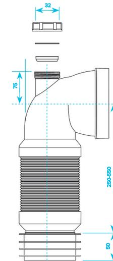
90° Flexible Pan Connector (32mm Adapter)
