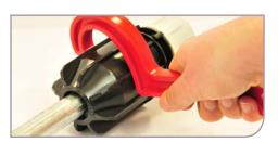
Tighten the black nut using a Plasson wrench or similar. Assemble the Metric PE joint as per the standard fitting instructions.
