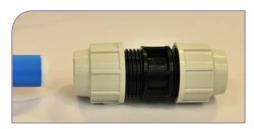
Insert liner into pipe (metric 20mm-63mm only) and slacken nut until half the thread is visible.
